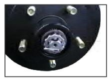
Install hub nose O-ring & adjust bearings per attached UFP Assembly Instructions.\*
