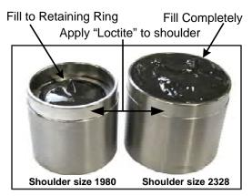
Fill THE VAULT protector cap with HYBRID-OIL lubricant. As shown in the photo above. Apply "Loctite" retaining compound to shoulder of protector.
