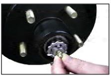
Screw a 1/16" NPT (Auto parts store) grease fitting into the threaded hole in the end of the spindle.
