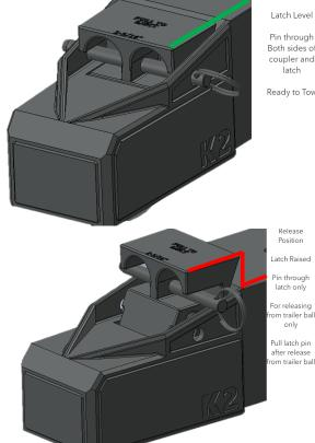
Caution - Failure to tow with the latch in down,
