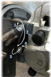
3) Feed one end of the remaining "U" up through the bottom fastener from 6 o'clock position to the 12 o'clock position. Feed the other side of the "U" along the right (clockwise) side of bottom bolt so both meet at the 12 o'clock position of bottom bolt.
